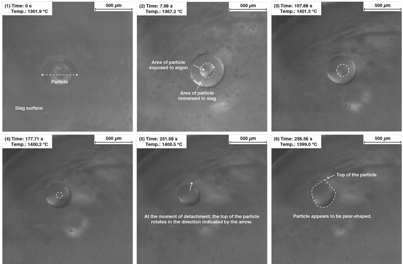
Fig. 2—A \text{MgAl}_2\text{O}_4 spinel particle detaching from the slag surface observed during the experiment.
